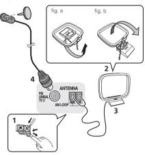
**1** Push open the tabs, then insert one wire fully into each terminal, then release the tabs to secure the AM antenna wires.
